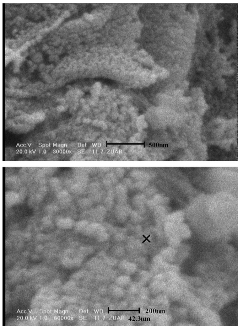
Fig. 2. SEM of the synthesized silica nanoparticles
